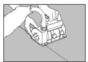
The sheets are hot welded. Do not weld until the adhesive has bonded completely, wait 24-48h. The joints are chamfered or grooved to about 3/4 of the thickness using a hand grooving tool or machine prior to welding.
